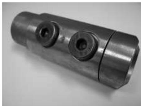
1.5 To bolt together, insert and tighten both bolts part of the way into their threads. Where multiple joints are fitted to a cage, ensure that all bolts have been fitted to all joints partially before you begin to tension any joints up. Warning: the threads are fragile and if damaged may require that section of cage to be replaced.
