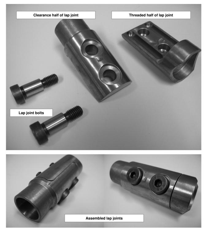
This can be done with a G clamp. DO NOT use a pry bar to align the joints - it may damage the threads. To bolt together, insert and start/tighten both bolts part of the way in to their threads. Start all of the lap joints (there will be 4, 6 or more, depending on the cage) by inserting all the bolts and starting/tightening loosely before any joints are tightened fully. Warning: the threads are fragile - carefully align both halves of the lap joint before carefully inserting the bolts.
