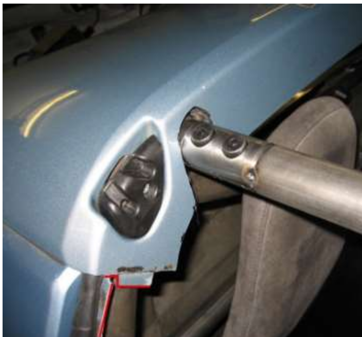
Figure 1. Rear hoop fibreglass trim
