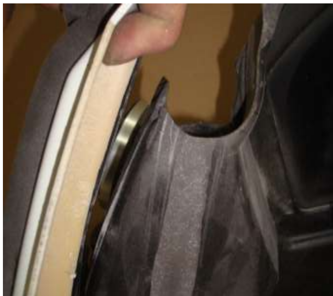
Figure 7. Outer skin separated from bulkhead panel
