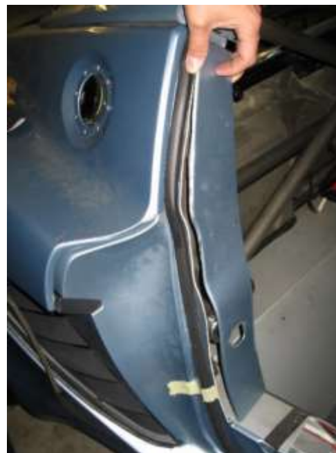
Figure 2. Door fibreglass trim
