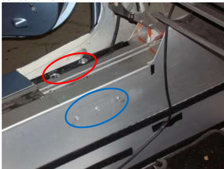
Figure 8. Trimmed sill trim with holes drilled
