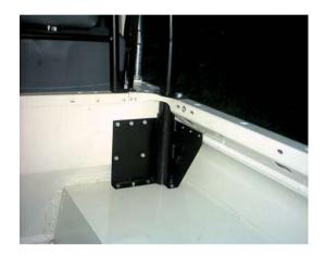
There are 2 brackets that sit inside the rear tub and should be dropped into position at this point - see assembly drawing and photo above for correct orientation of brackets. *If fitting to a non bulkhead vehicle then these brackets may not be compatible with the bulkhead replacement bar.*
