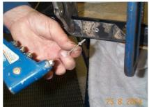
On the vehicle there is a lower flange that runs backwards under the doors. The top edge of this needs completely removing just rearward of the hole for the retaining strap. Cut flange away right back to hinge pillar. Leave 0.25" of the top of flange, i.e. cut 0.25" away from bend on top. Then cut corresponding material out of wing flange. Stand the chassis mount in position on the chassis outrigger
