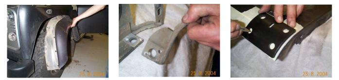
Mark holes in wing, drill out to 12mm and cut between them to create square hole.
