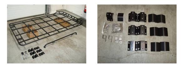
1.4 - The aluminium clamps and stainless brackets need to have the self adhesive rubbers applied to them at this stage.
