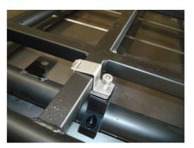
2.4 - Using the M8 x 16mm countersunk bolts and spring washers provided, attach the lower section of each clamp to the upper section. Copper grease should be applied to the threads to aid fitment. These should not be tightened fully at this stage.
